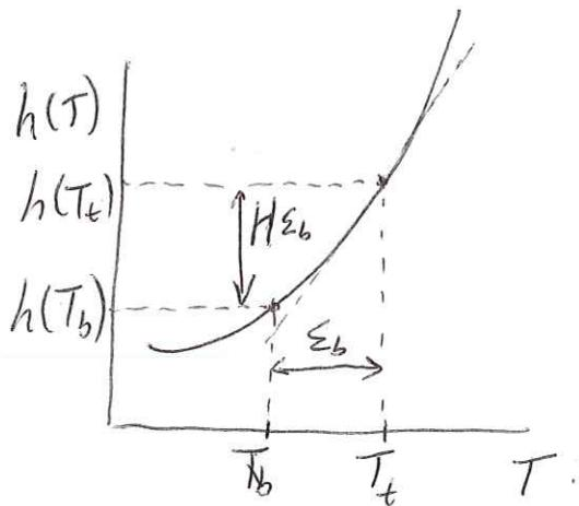
$$h(T_t) \approx h(T_b) + \left. \frac{\partial h}{\partial T} \right|_{T_b} (T_t - T_b)$$
