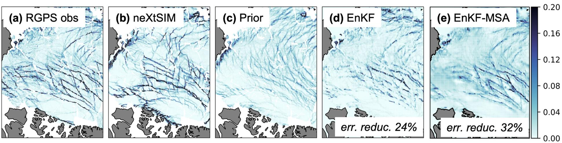
(a) Observed ice deformation from RADARSAT Geophysical Processing System (RGPS) satellite images, (b) neXtSIM simulation. neXtSIM simulation matches well the observed distribution and multifractal scaling of ice deformation.
