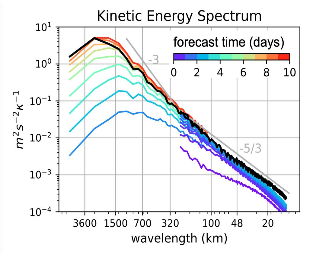
We characterised the wind uncertainties across scales based on ECMWF and AROME-Arctic ensemble forecasts. The kinetic energy spectra show wind errors at different forecast lead time (colored lines) and different spatial scales.
